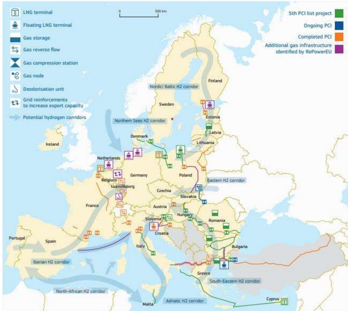
Fig 2. European gas infrastructure map – projects for common interest (PCIs) and additional projects identified through REPowerEU, including hydrogen corridors
